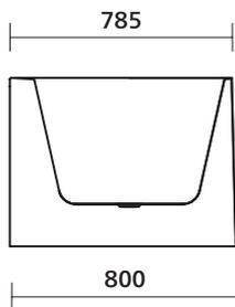
Leave a 3mm gap between base of bath and floor. Use silicone to seal base of bath to floor, leaving a 20mm weephole.
